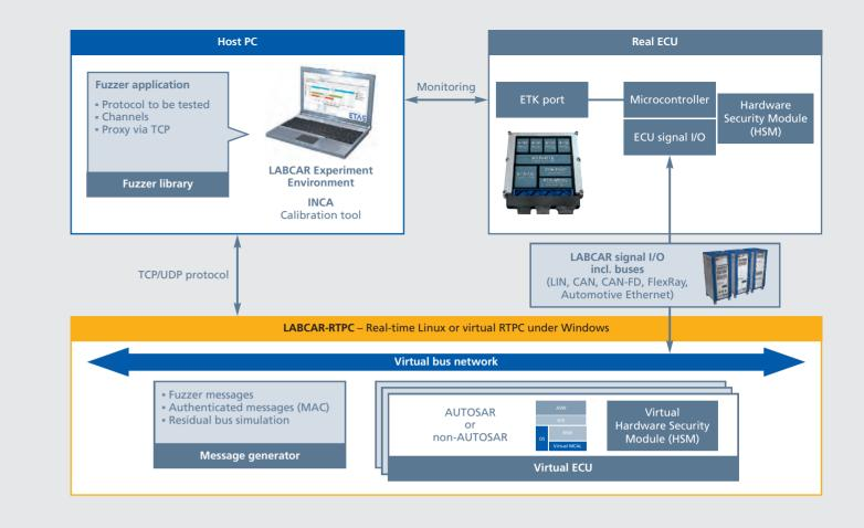
• Penetration (PEN) testing: testers attempt to manipulate the behavior of ECUs externally (for example, through human intervention), read out data without authorization, or corrupt the embedded system. To ensure ideal test coverage, the partially automated PEN Testing-in-the-Loop from ETAS and ESCRYPT utilizes an "attack library," which is continually being extended with experience gained from ESCRYPT consulting projects.
