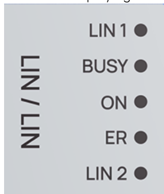
Fig. 2-2 LED layout of the ES134.1
