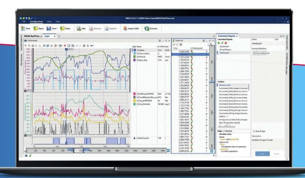
Using a search criterion defined as a calculated signal (right), the event list (center) allows users to navigate from one result to another. The selected signal is displayed in the virtual oscilloscope (left).
