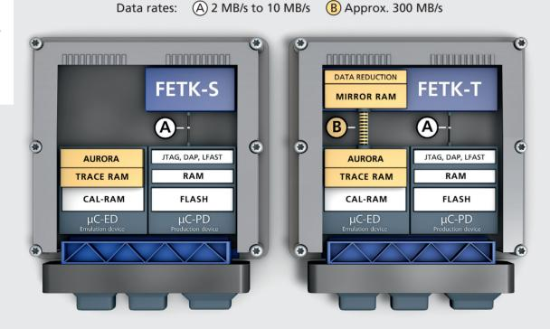
FETKs are available in two versions: FETK-S (left) and FETK-T (right). Both variants use a microcontroller-specific production device (µC-PD) debug interface such as JTAG (Joint Test Action Group), DAP, or LFAST as access to the ECU. The FETK-T version additionally supports the particularly powerful µC emulation device (µC-ED) trace interfaces together with the high-performance transmission of trace data from the ECU via the serial Aurora interface.
