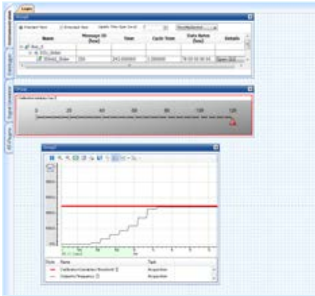
Image 5: Normal behavior of PWM over time. The red line represents the threshold (max 1,200Hz).
