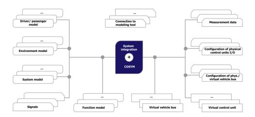
The various components of system simulation with ETAS COSYM.
