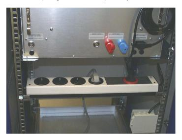
You can, for instance, make the signal box the master by plugging it into the red socket of the plug strip. When the master is switched on, this fact is detected by the plug strip. Consequently all the slave sockets are switched on via a bipolar relay. All devices connected to the slave sockets are now supplied with power. If the device connected to the master socket is switched off, all devices connected to the slave sockets are cut off from the power supply as well.
