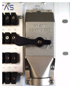
Fig. 3-2 Fixing the DLM5-260 Connector (Example)
