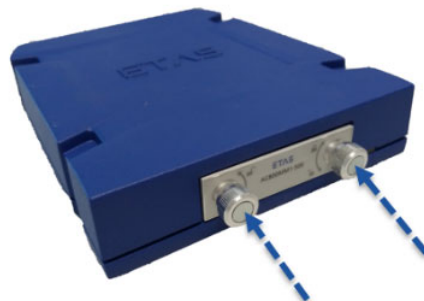
Fig. 4-2 Pushing in the pressure turn-lock fasteners
