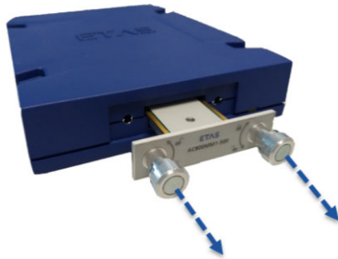
Fig. 4-5 Pulling out the memory module
