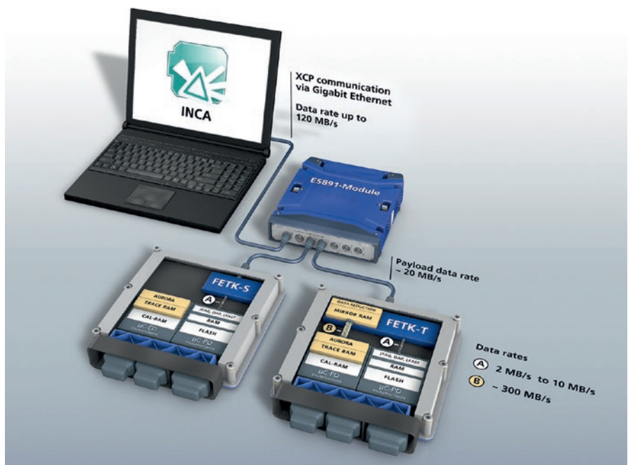
Gathering data from the ECU using the FETK interface: the FETK is offered in two versions, the FETK-S (below left) and the FETK-T (below right). Both versions use a microcontroller-specific debugging interface of production devices ( \mu C-PD) – for instance JTAG (Joint Test Action Group), DAP, or LFAST – to access the control unit (A). The FETK-T also supports the particularly powerful \mu C trace interfaces of emulation devices ( \mu C-ED), as well as transferring trace data from the ECU with great effectiveness using the serial Aurora interface (B).
