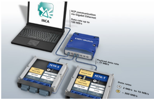
Figure 1: System view ECUs with FETK Interfaces communicate with the host application via an ES891 ECU and Bus Interface Module. In addition, measurement data from bus communication via CAN, FlexRay, LIN and measuring modules can be recorded by the ES891 module. It captures the signals from the connected source synchronously, bundles and transmits them to the host application, e.g. to ETAS INCA, as shown in the figure.
