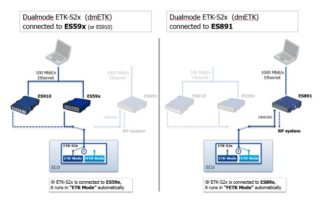
**Note:** The only possibility to connect an ETK-S2x to an ES89x is (as shown on the right side in the graph above) with the adapter cable CBAE360.1 (4 pin/10 pin) [F-00K-109-448].
