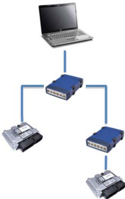
Figure 5: Connection set-up with two ETK ECUs connected to ES59x devices using the integrated Ethernet switch of one of the ES59x.
