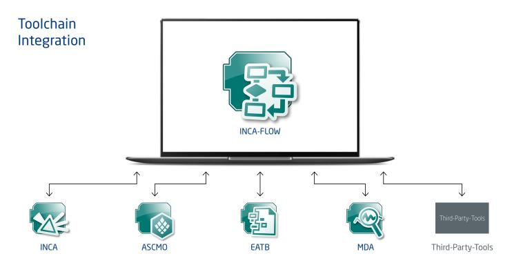
**INCA-FLOW and INCA:** Enables the automation of ETAS INCA for ECU access, signal measurement and calibration of ECU parameters.
