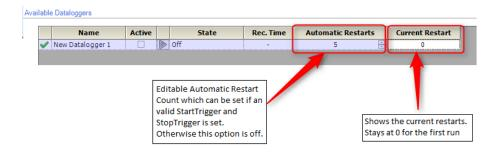
The "Automatic Restarts" feature is always coupled to a valid StartTrigger condition including a specified post trigger time or a
