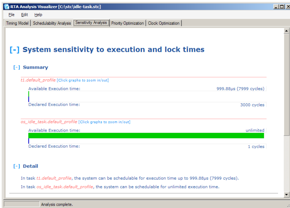
Figure 7.14: Sensitivity analysis for the idle mechanism
