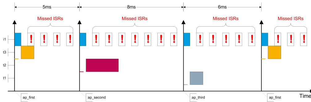
Figure 5.4: Missed profile releases with automatic inclusion of a coarse activator profile in a timeline transaction
