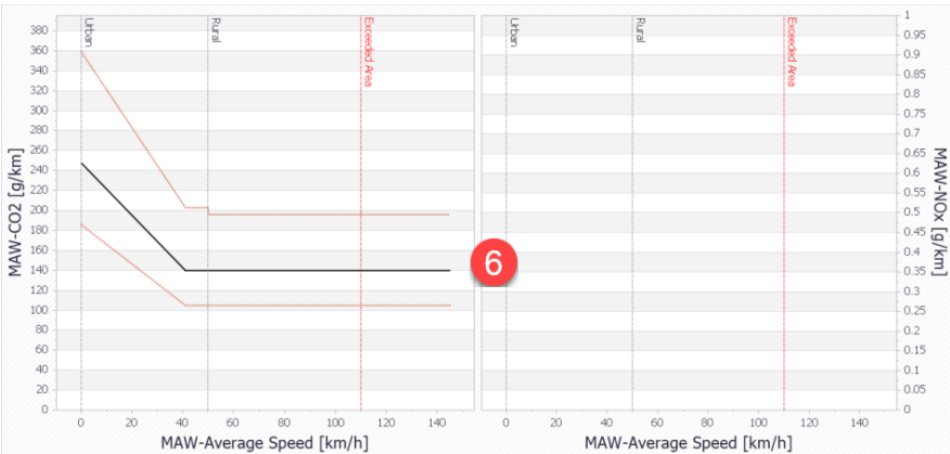
6: Instrument: Moving average window, MAW- CO2 and NOx diagrams
